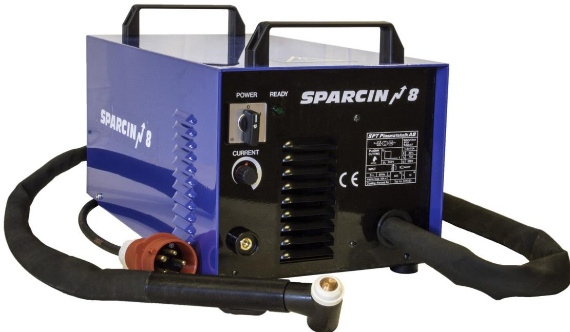
**SPARCIN 8** is a highly efficient multi-plasma system with water-cooled torch for all types of industrial plasma cutting and gouging up to 20mm.
